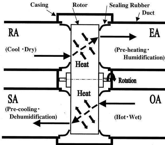
Figure 1 Both heat and moisture transfer through honeycomb.
