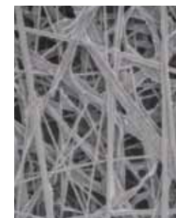
Picture 2 SEM picture of metal silicate before synthesization
